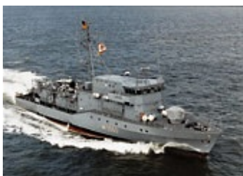
GERMAN minesweepers made of non-magnetic stainless
