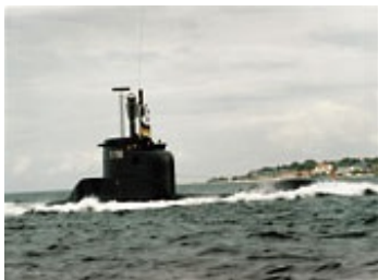
SIX NEW SUBMARINES are being made of an austenitic non-magnetic stainless steel containing 16% nickel
