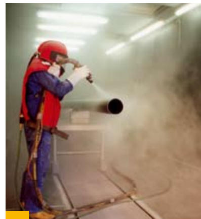
Glass marble peening improves the surface properties
