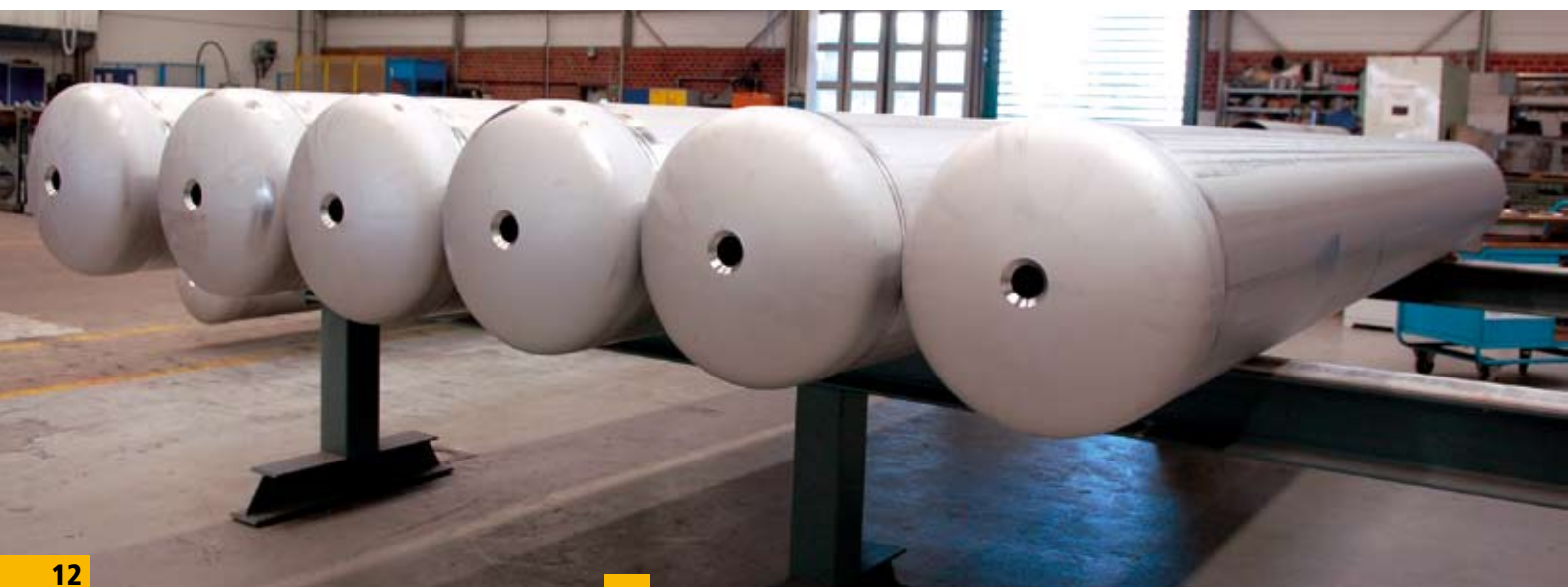
H 2 reservoir pipe with welded on dished end for HDW
